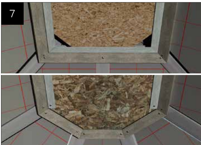
This is how battens should look round Georgian end (top) and Victorian end (bottom).
